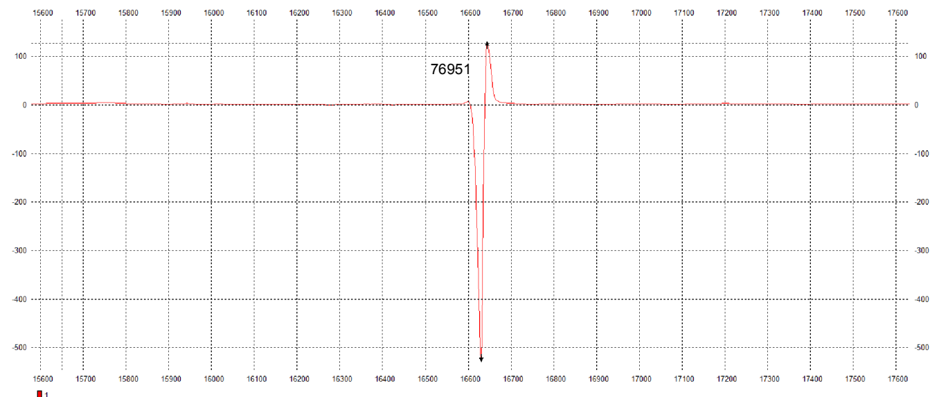
Magnetic profile of 76951 measuring 1,424 nT
